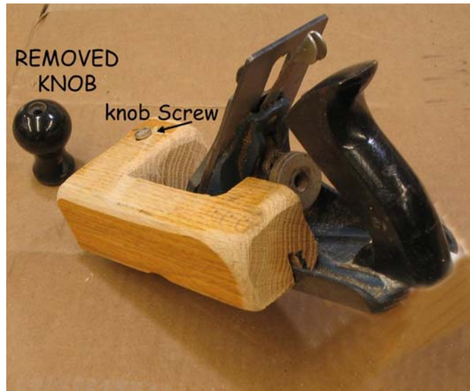
Figure 2. “Hot Dog” accessory Tote for Shooting Attached to a Stanley #4 Bench Plane
